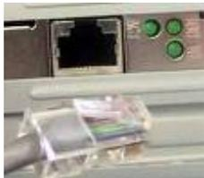
The easiest way to confirm whether or not you have a network connection, is to look at the back of your computer. The network port, pictured on the right (probably the only port with lights) should have a cable going into it, and the lights should be flashing. If the lights are flashing, you will need to ring the help desk for them to look at your login.
