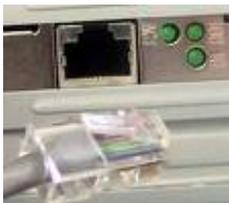
Network cables go from the wall (normally) to the back of your computer. Check on the back of your computer to see if the cable is plugged in. Network ports have lights on them. If the lights are flashing, you know that the cable is connected properly. If there are no lights, push the cable in at both the computer and wall, to ensure a secure connection.
